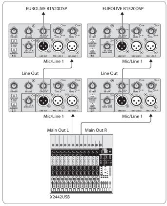
Fig. 4.3: Linking several B1520DSP speakers
